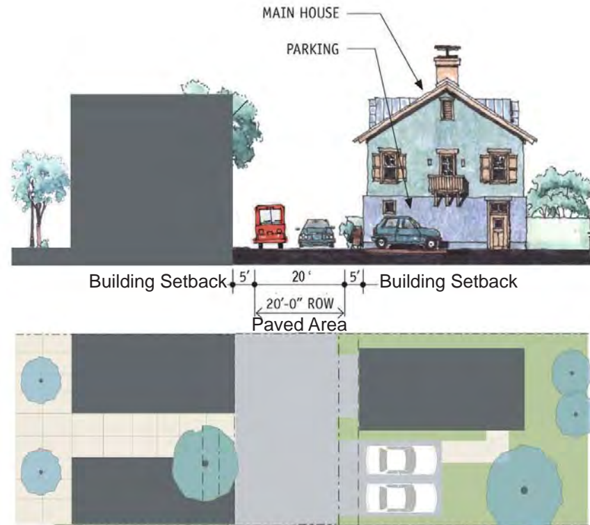
EXHIBIT 10.23 – TYPICAL COMMERCIAL ALLEY CROSS SECTION
